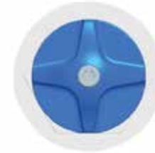
**Low-speed compression** adjustment is useful to control fork performance during rider weight shifts, G-outs, and other slow inputs.
