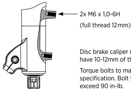
Disc brake caliper mount bolts must have 10-12mm of thread engagement. Torque bolts to manufacturer's specification. Bolt torque must not exceed 90 in-lb.
